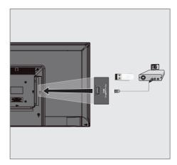
Connect the »USB« interface of the television and the corresponding socket on the data device (external hard disk, digital camera, card reader or MP3 player) using a USB cable.
