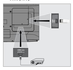
Plug the external hard disk to the USB2 (HDD) USB interface of the television;
