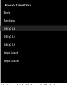
12 Select »DiSEqC1.0« or »DiSEqC1.1« according to your current antenna type and confirm with » • «.
