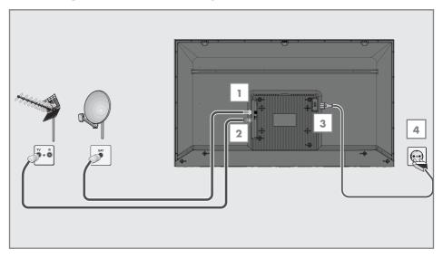
To receive digital satellite channels (DVB-S), connect the satellite antenna cable to the **»SATELLITE**« antenna socket on the television set;
