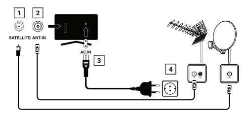
For digital satellite stations (DVB-S/ S2) plug the cable of satellite antenna into the antenna socket SATELLITE on the television set;
