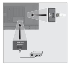
Plug the external hard disk to the USB2 (HDD) USB interface of the television;
