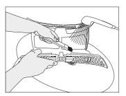
• Insert the fibre filters on one another and place it back in its place.
