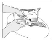
• Clean both filters under water running in reverse direction of fibre accumulation or with a soft brush. Dry the filter before placing it back.
