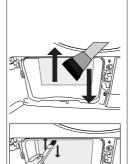
Clean the fibre on the metal surface of the condenser with damp cloth or the brush on the air deflector in up - down direction. Do not clean with left - right direction since it will damage the metal plates of the condenser.
