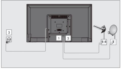
For digital satellite stations (DVB-S/S2) plug the cable of satellite antenna into the antenna socket **RF IN-S2** on the television set;
