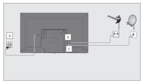
1 To receive digital satellite channels (DVB-S), connect the satellite antenna cable to the »SATELLITE« antenna socket on the television set;
