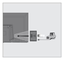
1 Connect the USB interface of the television and the corresponding socket on the data device (external hard drive, digital camera, card reader or MP3 player) using a USB cable;
