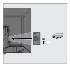
Plug the external device to the **USB1** or **USB2** USB interface of the television;
