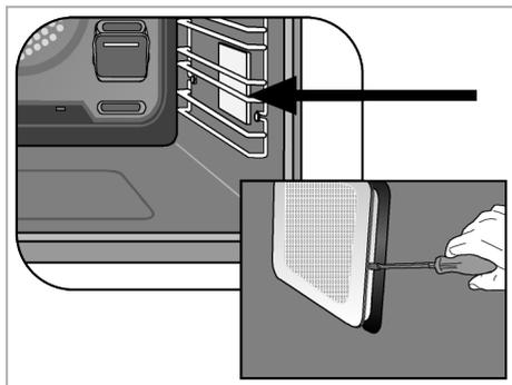
3. Lift the lamp's protective glass cover with a screwdriver. Remove the screw first, if there is a screw on the square lamp in your product.
