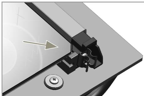
The first step of regrouping the door is to replace the second and third glasses (2, 3). As shown in the figure, place the bevelled edge of the glass to meet the bevelled edge of the plastic slot.
