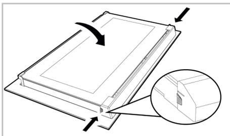
2. Pull the plastic component, attached on the upper section of the front door, towards yourself by simultaneously pushing on the pressure points on both sides of the component and remove it.
