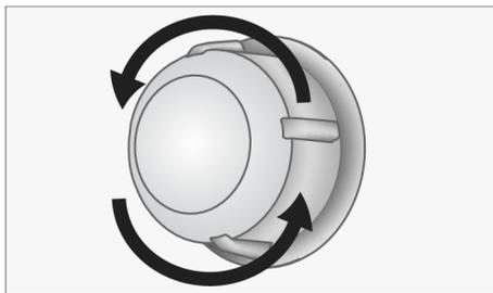
3. If your oven lamp is type (A) shown in the figure below, rotate the oven lamp as shown in the figure and replace it
