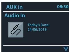
In AUX in mode plays audio from an external source. Turn the volume low on both the radio and, if adjustable, the audio source device. Enter AUX mode, then adjust the volume as required.
