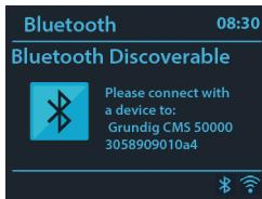
In Bluetooth mode, you can turn on the Bluetooth of your Bluetooth device. Press and hold »**BTPAIR**« to turns Bluetooth discoverable. From your Bluetooth device, search the HiFi System Grundig DTR 7000 to pairing. When it is waiting for pairing, there is a blinking Bluetooth icon at the bottom. If the pairing is successful, the Bluetooth icon becomes steady. Control the music playback from your Bluetooth device.
