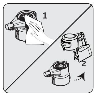
Install the metal filter inside the dust container (11) by rotating it clockwise.
