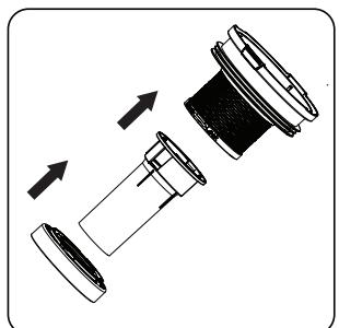
Once dry, push the cyclone cone in the direction of the arrow and fix it together.
