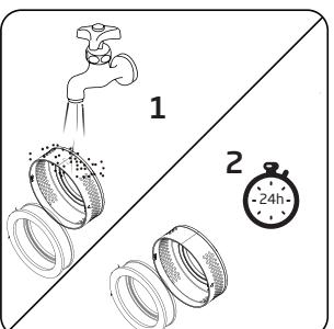
Gently shake the exhaust filter to clean the dust, wash it under running water for and leave it to dry for at least 24 hours.
