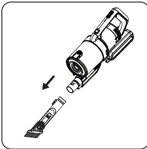
Attach the narrow mouth nozzle **L** to the opening of the body. To remove the narrow mouth nozzle, press the eject button to remove it.
