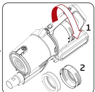
Remove the exhaust filter cover by turning it in the direction of the arrow.
