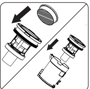
Install the motor input filter to the cyclone cone and place it into the dust reservoir.
