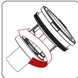
Remove the cyclone cone by turning it in the direction of the arrow and remove the dust on it.
