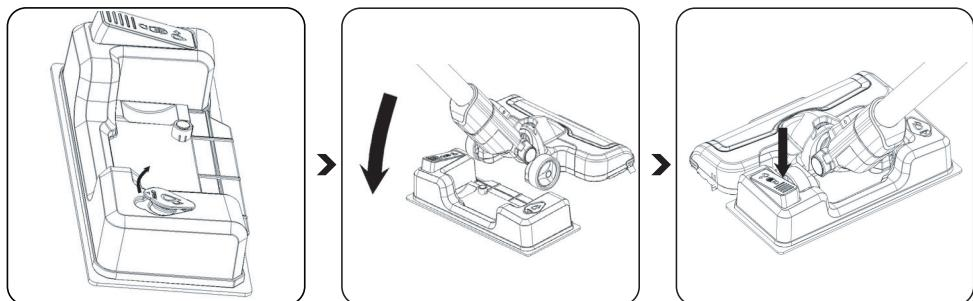
Open the water tank **N** cover in the direction of the arrow, fill the water tank with the help of a glass or faucet.
