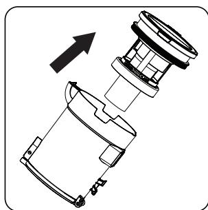
Remove the cyclone cone from the dust container.
