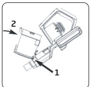
To attach the dust container to the body, place the dust container locking tab into the slot inside the body.
