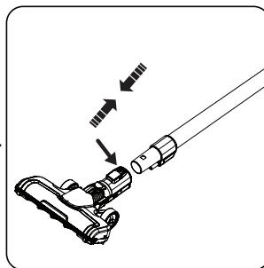
Attach the electric turbo brush **[J]** to the tube **[H]**. Remove it by pressing the turbo brush release button **[I]**.
