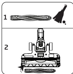
To clean the dust on it, gently hit on a hard surface to allow the dust on the brush pours out. Or, remove the dust from it with the help of a brush.
