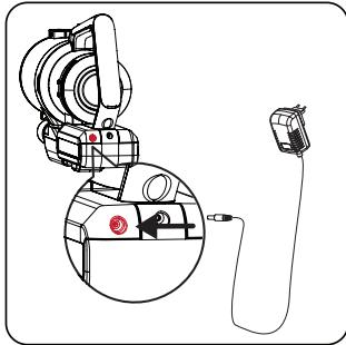
Plug one end of the adapter [K] into the outlet and the other end into the charging slot, which also has a body.
