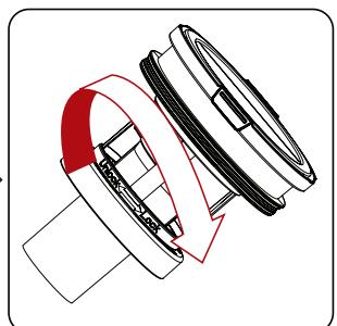
Turn the cyclone cone in the direction of the arrow and replace it.
