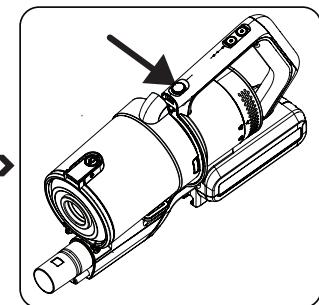
To clean the cyclone cone in the dust container, press the dust container removal button **E**.
