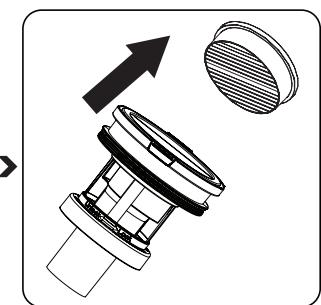
Remove the motor input filter from its holder and remove it in the direction of the arrow. Remove the dust accumulated in the motor input filter before washing. To remove dust from the motor input filter, you can pour the dust by gently hitting it on a hard surface. Or, you can clean the dust from the motor input filter with the help of a brush.
