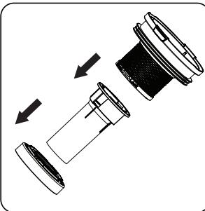
Remove the cyclone pipe and its holder.
