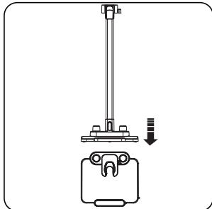
Place the charging station **[Q]** onto charging station support **[P]**.
