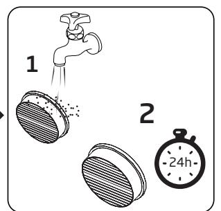
Wash the motor inlet filter under running water and leave to dry for 24 hours after gently squeezing it.
