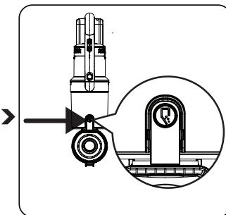
Remove the metal tube **H** from the body.
