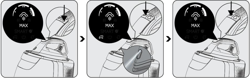
Set the fabric-appropriate temperature and steam using the level adjustment button (3). (See 3.6)
