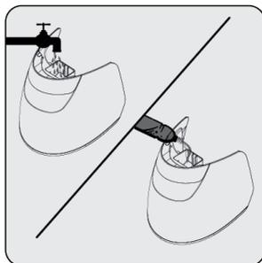
Fill the water tank (11) up to Max line.
