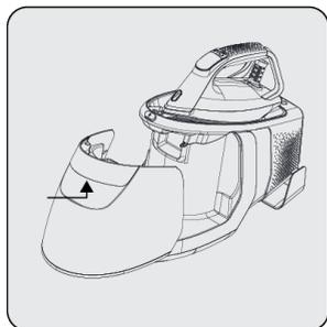
Remove the water tank (11) by holding it from the tank detachable handle (13) and pulling.
