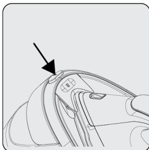
To detach the iron from the dock, push on the carrying lock unlock button (14).
