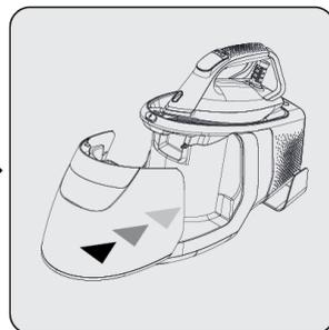
Place back the water tank (11). Make sure the water tank is properly seated.
