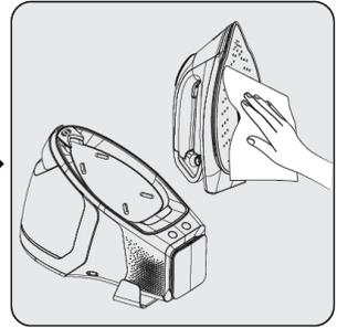
Use a damp cloth to clean the outer part of the appliance. Then wait for it to dry completely. Wipe the sediments and residues on the soleplate (16) with a lightly dampened cloth.
