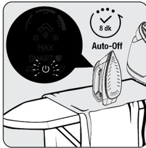
Iron will automatically turn off if it does not move vertically for 8 minutes or any buttons are pressed.
