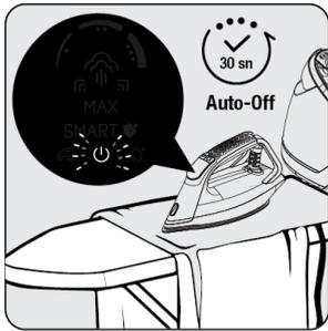
Iron will automatically turn off if it does not move horizontally for 30 seconds or any buttons are pressed.
