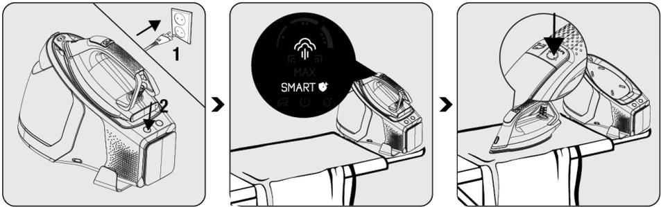
Plug in the power cord and press the on/off switch.
