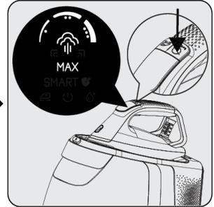
Push the level adjustment button (3) and hold for 3 seconds.
