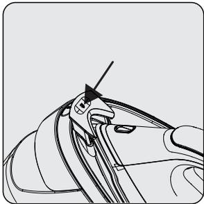
Place the iron on the dock (10) and push on the carrying lock (15) to lock the iron.
