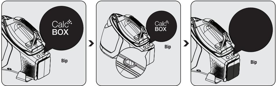
The calc cleaning button “Calc<sup>+</sup> BOX” (5) will remain lit for 20 seconds and alerts with a “beep” sound. This indicates the time for calc cleaning.
