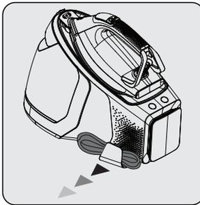
Pull the steam cable clip (9) and place the cable.
