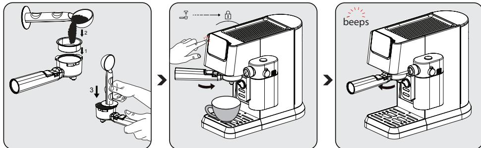
Place the single or double espresso basket into the filter holder. Fill the freshly ground coffee powder into the filter with measuring spoon (approx. 8-15g) and use the spoon to flatten the excess powder. With the tamping end of the spoon, apply around 15 kg to push down the powder even and firmly.
