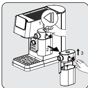
Holding the milk tank with one hand, press the button on the top of the milk tank lid to remove the milk tank rightwards. Remove the lid of the milk tank by pressing the release button on the right side of the lid body.
