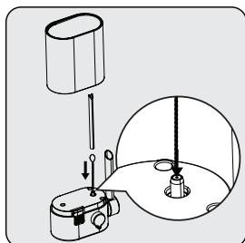
Use the cleaning needle (15) to clean inside the milk frother inlet.
