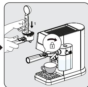
Insert the single basket into the portafilter. Fill the filter with finely ground espresso powder (approx. 8-15 g). Press the powder down with the flat side of the coffee spoon. Install the portafilter under the coffee outlet. Align it with the unlock symbol, slide it into the groove, and slowly rotate it to the right to the lock symbol.
