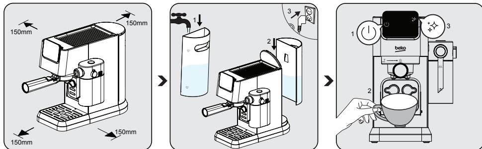
Choose a safe and stable surface with an easily reachable power supply and allow the minimum distance from the sides of the machines.
