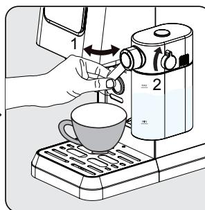
Add milk to the milk tank. The milk should always be below the max mark. The recommended temperature for milk is 4-8 °C (~ 40-46 °F). Put on the lid of the milk tank and attach the milk tank to the appliance, it must click audibly into place. Make sure that the milk tank fits correctly. Adjust the angle of the milk foam outlet over the cup. Adjust the milk foam density with the help of knob based on your preferences.
