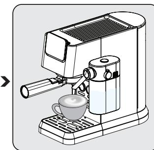
The pump will work intermittently as the milk froth first enters your cup. After the milk froth is ready, the device automatically starts to brew the coffee.
