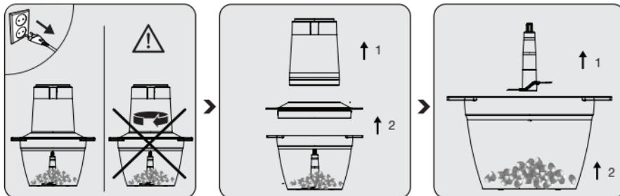
When the operation is completed, stop pressing the operation button. Unplug the appliance and wait until the blade is completely stops.
