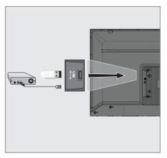
1 Plug the external hard disk to the **USB** USB interface of the television.
