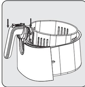
There are 2 notches on both sides of the handle. Lock the basket in the drawer by sliding the tabs into the notches on the top of the basket drawer.
