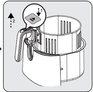
To release the basket from the drawer, place the drawer on a flat surface. Lift the protection cover (5), press the basket release button (6) and lift the basket out of the drawer.
