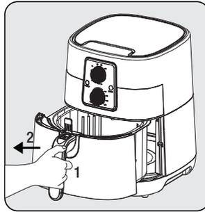
Firmly grasp the removable basket handle (7) to open the basket drawer; then remove the drawer from the machine.
