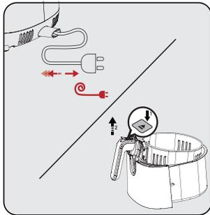
You can pull and release the cable (11) to store it in the cable storage area. Press the basket release button (6) and remove the removable basket (9) by lifting and pulling the handle (8) upwards.
