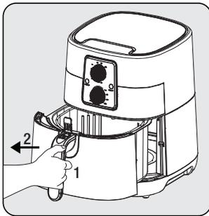
Firmly grasp the removable basket handle to open the basket drawer; then remove the drawer from the appliance and place it on a flat and clean surface.
