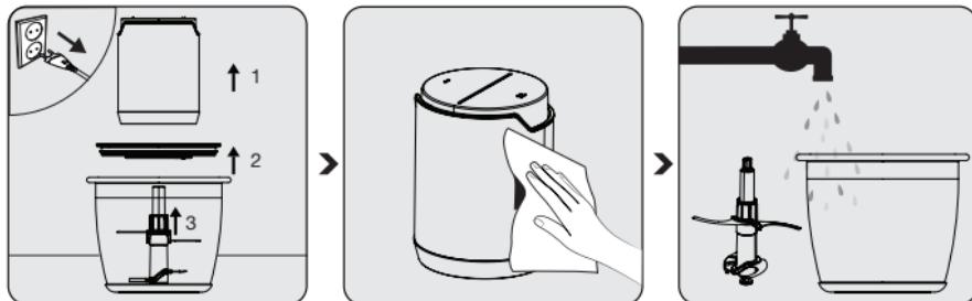
Unplug the appliance. Remove the motor unit (4), spacer lid (3) and then the blades (6).
