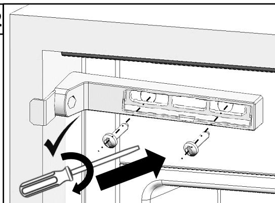
*Installation step for 14\_2: screws should not be fully tightened at this stage.*
