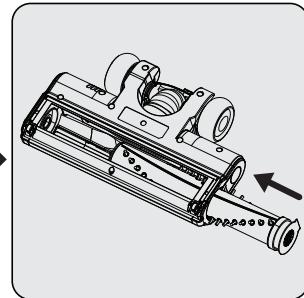
Fix the roller back to its place by pushing.
