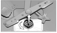
Pull out the metal/plastic filter (3) from the seating.
