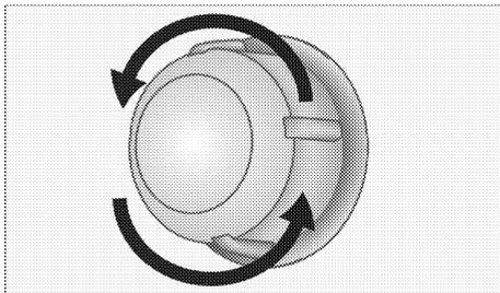
3. If your oven lamp is of type (A) shown in the figure below, remove it by rotating as shown and replace it. If it is of type (B), pull and remove it as shown in the figure and replace it.
