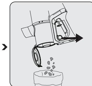
Pull the emptying dust container ring (4) to the last point. Dust container lid will be opened. Empty all the dust it contains.
