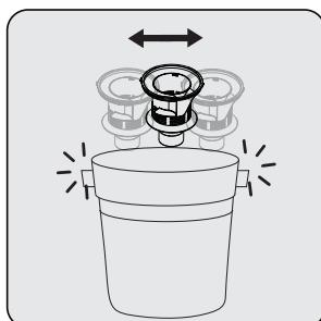
Remove the dust on the plastic filter by tapping it on a hard surface such as a waste bin or by using a brush.
