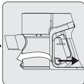
For a detailed cleaning of filters, remove the dust container by turning it clockwise while pulling dust container ring (4) lightly.
