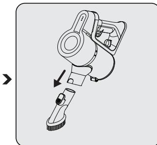
**Dust brush (14):** Suitable for vacuuming curtains, waxed furniture and delicate and fragile objects.
