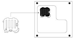
Tilt the machine back slightly. Rest the tabs of Cover A against the lower panel. Complete the assembly by rotating the cover.
