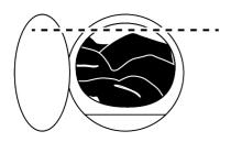
In the 6 kg Washing and 6 kg Drying programme, it is recommended to fill the machine to the level shown in the figure above for ideal drying conditions (you can see the level arrow when you open the loading door).
