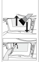
Clean the fibre on the metal surface of the condenser with damp cloth or the brush on the air deflector in up - down direction. Do not clean with left - right direction since it will damage the metal plates of the condenser.
