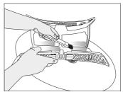
Clean both filters under water running in reverse direction of fibre accumulation or with a soft brush. Dry the filter before placing it back.
