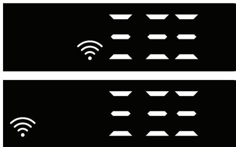
The display when HomeWhiz is enabled. If you press the remote control key while the function is enabled, the Home Whiz function will be disabled, and the product indicator will return to the delay time/ programme time display. In the off position, the HomeWhiz key LED will go off. To switch off the wireless connection function, press and hold the Remote Control Key for 3 seconds while the product is on. After the 3 - 2 - 1 countdown on the display, the wireless connection function will be
