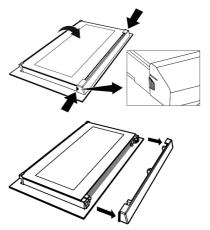
As shown in the figure, gently lift the innermost glass (1) towards "A" and then, remove it by pulling towards "B".
