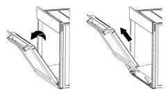
Pull the removed door upwards to release it from the right and left hinges and remove it.
