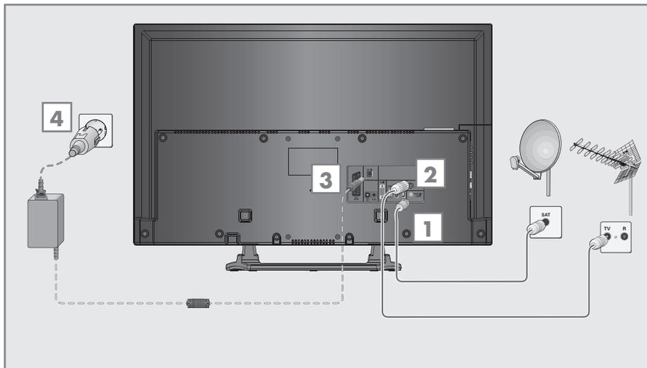
**1** To receive digital satellite channels (DVB-S/S2), connect the satellite antenna cable to the antenna socket »**SATELLITE**« on the television set.
