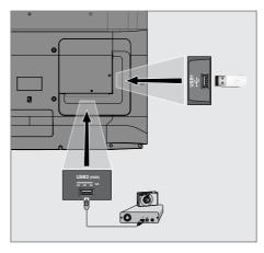
Connect the USB2 (HDD) interface of the television and the corresponding socket on the data device (external hard drive, digital camera, card reader or MP3 player) using a USB cable:
