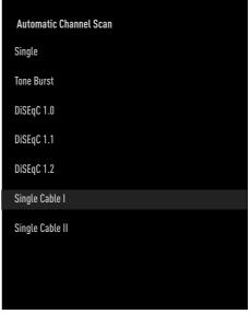
12 Select »Single Cable I« or »Single Cable II« according to the type of single cable router multi-switch in your antenna system, and confirm with » • «.
