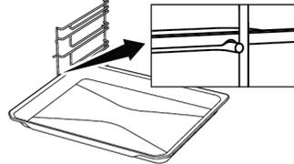
**Proper placement of the wire grill and tray on the telescopic rails-On models with wire shelves and telescopic models**
