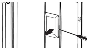
3. Lift the lamp's protective glass cover with a screwdriver. Remove the screw first, if there is a screw on the square lamp in your product.
