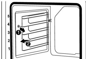
3. To reattach the shelves, the procedures applied when removing them must be repeated from the end to the beginning, respectively.
