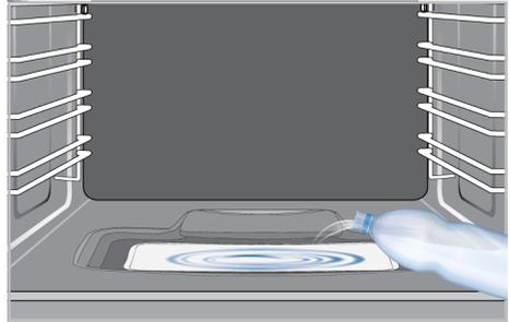
2. Wait at least 30 minutes to allow the vinegar to dissolve the lime residues at ambient temperature.
