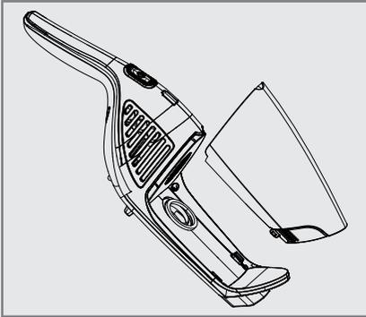
2 Pull the filter from its holder by holding the handle and remove it from dust container **I**.
