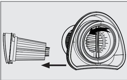
4 Wash out the dust container **I**, filter holder and HEPA filter under the running water.
