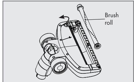
2 After cleaning and drying the brush roll, reattach it and lock the tab.
