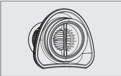
3 Remove the HEPA filter by grasping the handle of the filter holder and turning counter-clockwise.
