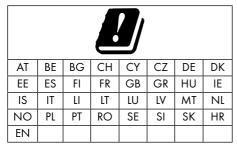
The 5150-5350 MHz band is restricted to indoor use only. (For Wi-Fi/Bluetooth built-in model or Wi-Fi Built-in model).
