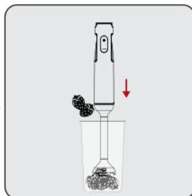
Put the ingredients (in small pieces) to be processed into the scale bowl (10) or the bowl that you will use and immerse the blending shaft (12) into the bowl.
