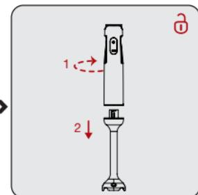
Turn the blending shaft (12) clockwise "②" to detach it from the motor unit (4).
