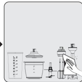
Unplug the appliance before cleaning. Make sure that all appliance components has stopped completely. Wipe the motor unit (4) of the appliance with a damp cloth.
