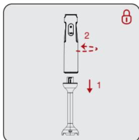
Attach the blending shaft (12) to the motor unit (4) by turning the end of the motor unit (4) "①" counterclockwise.
