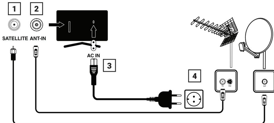
**1** For digital satellite stations (DVB-S/ S2) plug the cable of satellite antenna into the antenna socket **SATELLITE** on the television set;
