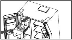
To remove the ice storage bin: Grab the handle on the bottom of the bin and pull it towards yourself. To reinstall the ice storage bin:
