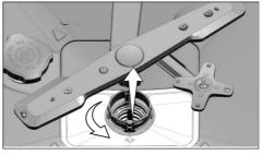
Pull out the metal/plastic filter (3) from the seating.
