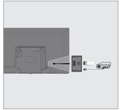
Plug the external hard disk to the USB USB interface of the television;
