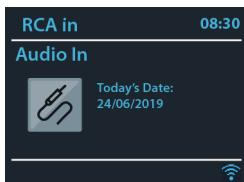
In RCA in mode plays audio from an external source. Turn the volume low on both the radio and, if adjustable, the audio source device. Enter RCA mode, then adjust the volume as required.
