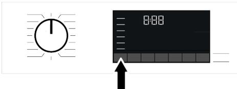
Whenever a new programme is selected, the recommended temperature for the programme appears on the temperature indicator. It is possible that the recommended
