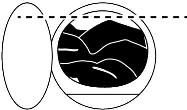
In the 6 kg of Washing and 6 kg of Drying programme, it is recommended to fill the machine to the level shown in the figure
