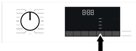
When you select a new washing program, press the Auxiliary Function Selection button to set the drying option suitable for this program.
