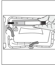
Pull the brush to the left to remove it. You can use the cleaning brush to clean filter, condensing metal surface and accumulated fibre on the door.
