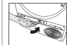
After the cleaning process is completed, place the air deflector cover to its place, move the latches to close it and close the toe board.
