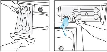
If fibre is accumulated in the funnel on the water tank, remove it under running water. Place back the water tank.
