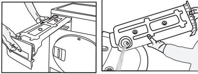
If fibre is accumulated in the funnel on the water tank, remove it under running water. Place back the water tank.
