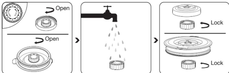
Turn over the lid **C** and open the backflow prevention cap by turning it anti-clockwise to remove it from the lid **C**.
